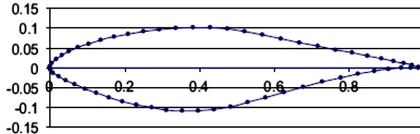
Fig. 1. S809 airfoil profile (unit: m).
